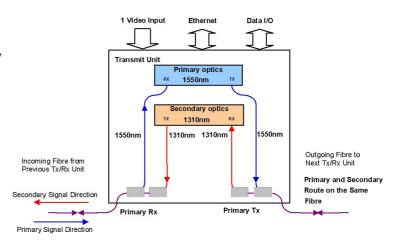
The **AMG3713E-DR-SF** receives and drops off data and Ethernet signals transmitted from an **AMG3784EN-DR-SF** receiver. It then inserts video, data and Ethernet signals onto the outgoing optical signal.
