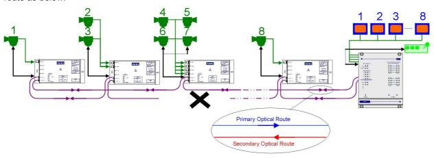
If multiple breaks occur, operation is maintained with all the units still physically connected to the receiver. For the scenario shown below camera signals and control would now be lost from cameras 1, 2 and 3 as there is now no physical connection between the transceivers and the receiver. However operation of cameras 4,5,6,7 and 8 remains fully functional.
