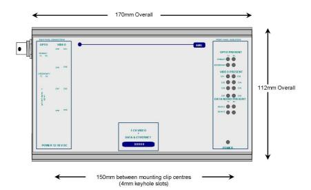
The **AMG3713E-DR-SF** is a standalone single channel video insert unit designed to transmit 1 video signal onto a singlemode optical fibre ring with Dual Redundant operation. It also provides one bidirectional data channel via a low speed data interface plus full duplex 100BaseT Ethernet connectivity around the ring..
