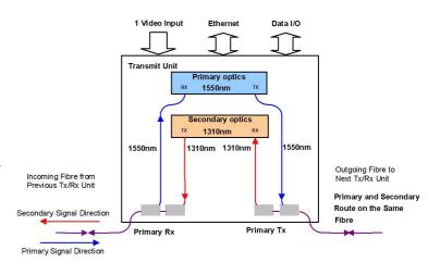
The AMG3713BxE-DR-SF receives and drops off data and Ethernet signals transmitted from an AMG3788BEN-DR-SF receiver. It then inserts video, data and Ethernet signals onto the outgoing optical signal.
