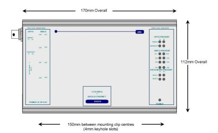
The **AMG3713BxE-DR-SF** is a standalone single channel video insert unit designed to transmit one video signal onto a singlemode optical fibre ring with Dual Redundant operation. It also provides bidirectional data channels via a low speed data interface, plus full duplex 100BaseT Ethernet connectivity around the ring.
