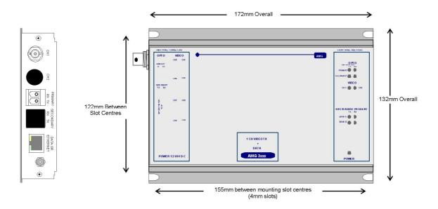
The **AMG3713-DR-SF** is a standalone single channel video insert unit designed to transmit one video signal onto a singlemode optical fibre ring with Dual Redundant operation. It also provides one bidirectional data channel via a low speed data interface.
