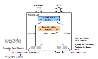
The **AMG3713-DR-SF** receives and drops off data signals transmitted from an **AMG3784-DR-SF** receiver. It then inserts video and data signals onto the outgoing optical signal.
