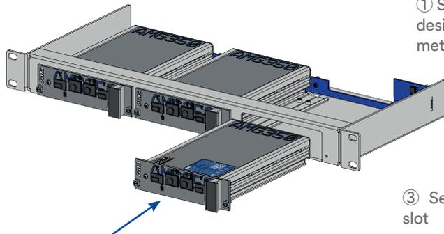
① Slide the unit into the desired slot using the metal guides as shown.
