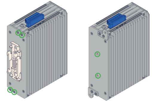
To maintain the units IP40 rating any screw holes that are not used should still have their screws installed as shown in green above.
