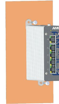
③ Fix the unit to the surface using two appropriate screws (screws not provided)
