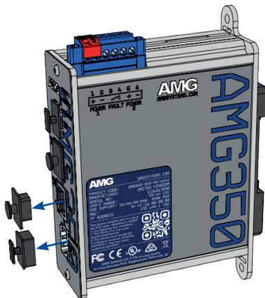
① Remove the dust caps from the RJ45 and SFP ports of the channel that is to be connected.
