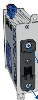
① Remove DIN rail clip by unscrewing the two fixing screws as shown.
