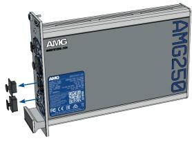
(1) Remove the dust caps from the RJ45 and SFP ports of the channel that is to be connected.
