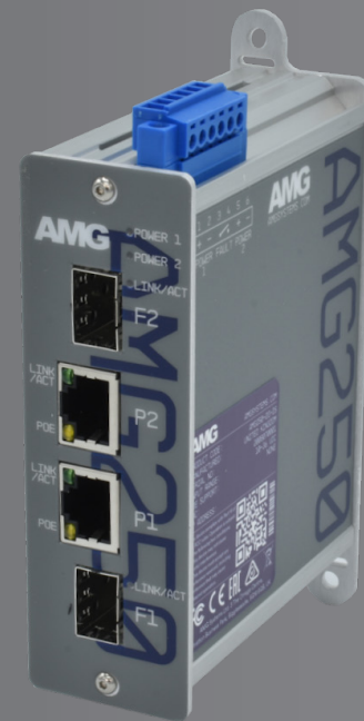
AMG250 2-2 Dual Channel Industrial Media Converter
