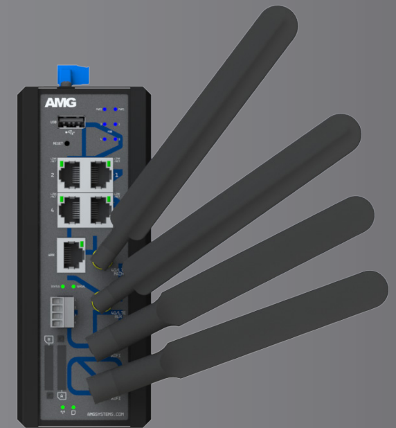
AMG750 Angled Antenna Industrial Grade Managed 4G Router
